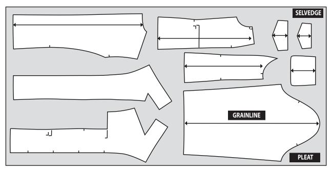
**FABRIC LAY PLAN** Please note: the lay plan is a suggestion and dependent on the width of fabric. This lay plan was created on fabric mt. 1.40 wide folded in double.
