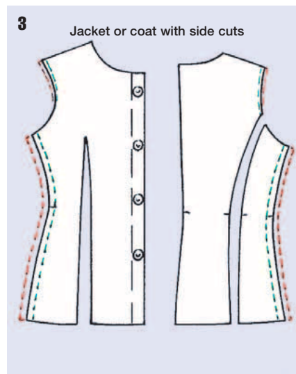
Figure 3 and 4 Dresses, blouses, jackets, coats: 1 cm at the side + 0.3 on the sleeve cap length. If necessary 0.5 cm on waist height.
